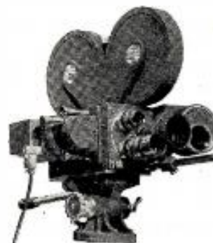
THE MAURER 16MM. , designed specifically for professional use, equipped with precision high-power focusing and view-finder. Standard equipment includes: 235° dissolving shutter, automatic fade control, view finder, sunshade and filter holder, one 400-foot gear-driven film magazine, a 60-cycle 115-volt synchronous motor, one 8-frame handcrank, power cable and a lightweight carrying case.
